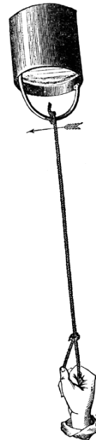
Figure 20.2: A bucket of water being spun in a vertical circle. Inertia (sometimes thought of as a fictitious “centrifugal force”) keeps the water in the bucket, even when upside-down. (Ref. [18]).
